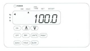
AFTER A FEW SECONDS THE SCALE WILL LOCK ON THE PERSONS WEIGHT, THE PERSON CAN NOW STAND OFF THE SCALE AND THE WEIGHT WILL REMAIN
